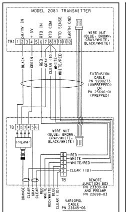
FIGURE 2-26. Wiring Model 396VP and 398VP to Model 2081 through a Remote Junction Box
